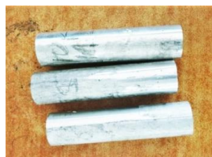
Fig.16:- After Machining The AlZrO 2 Pieces
