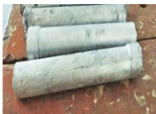
Fig.15:- Before Machining The AlZrO 2 Pieces
