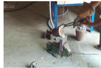
Fig11:- pouring molten metal into mould cavity
